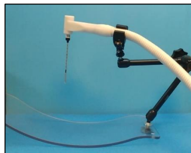
Fig. 3: Holder clamp positioning on the hose
